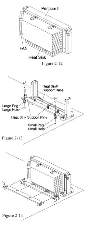
1. Finds out the Heat Sink Support (HSS) Mounting Holes on HOT-679 main board. Notice that one hole is larger than the other hole.
