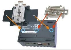
For DIN-rail mounting of the Edge-PC SPCEL12, the clip can be mounted in different alignments as required. Use the enclosed screws for mounting.
