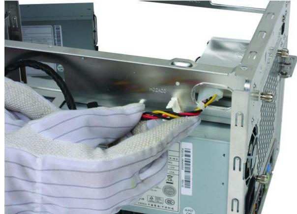
② Feed the HDD cable through the reverse hole as shown and attach to storage devices.
