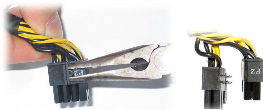
The ATX12V plug of the power supply consists of two 4-pin plugs, which can be combined to one single 8-pin plug. They can easily be separated again by using long-nosed pliers (as shown in the photo).
