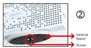
Unscrew one screw of the stand mount and remove the vertical stand.
