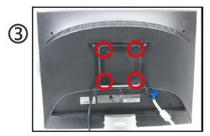
Fasten the VESA MOUNT at rear of LCD monitor with four screws.
