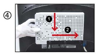
As shown, install the XS35 in the VESA MOUNT and push it towards the direction as indicated by the red arrow.
