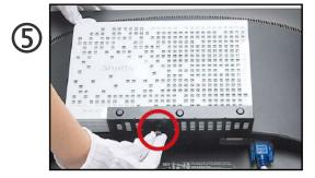
Check that it is properly aligned, then tighten securely with one thumbscrew.
