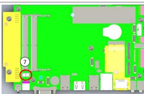
Connect the internal cable of PDC01 [6] to the onboard header [7].
