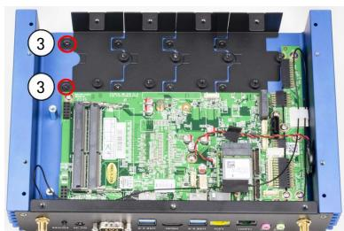
It is recommended to install this optional expansion kit from leftmost position. Undo two black screws [3] to remove a Dummy Bracket on the left side.
