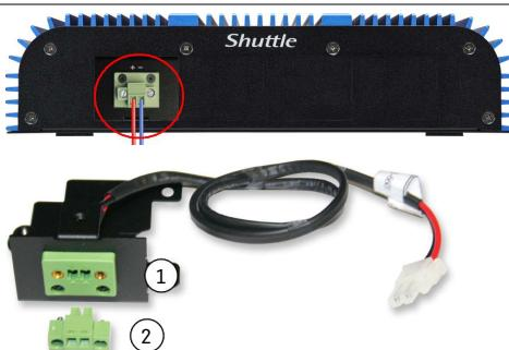
Connect the external cables of the power source to the terminal block [2] and fix it to the PDC01 [1]. The external cables are not included.
