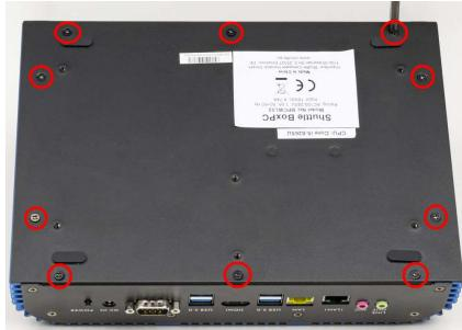
Unscrew ten screws of the base plate and remove it.
