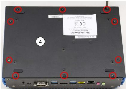
Unscrew ten screws of the base plate [4] and remove it.
