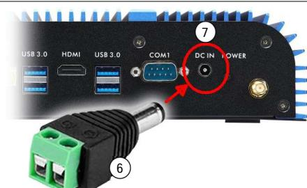
Plug the supplied adapter [6] into the DC input of the Box PC [7] if you require a screw terminal.
