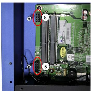
Take the VOL01 daughterboard [1], remove the protective film from the thermal pad [2]. Connect the VOL01 daughterboard to the onboard connectors of the mainboard [5] and fix it with two silver screws [3].
