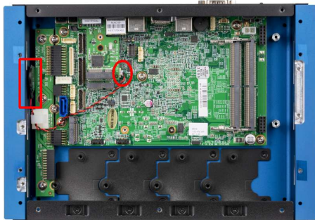
Photo: Position of the button cell battery and the connector on the mainboard with the computer housing open.
