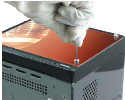
Align and correspond the transparent glass and new image to screw holes on the front of the machine.
