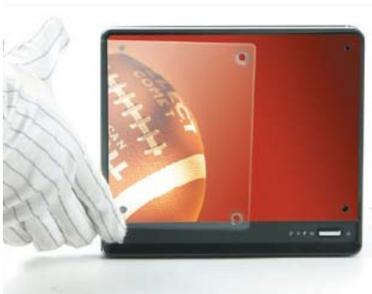
Insert the new image and cover back the transparent glass on top.
