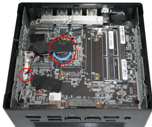
Photo: Position of the button cell battery and the connector on the mainboard with the computer housing open.
