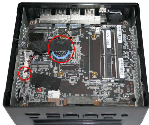
Photo: Position of the button cell battery and the connector on the mainboard with the computer housing open.
