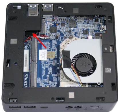
Photo: Position of the button cell battery with the computer housing open. (on the top of the housing)
