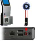
If, because of space constraints (e.g. in case of fixed installation), the machine cannot be switched on by pressing the front power button, it can be powered on by a separate remote line.
