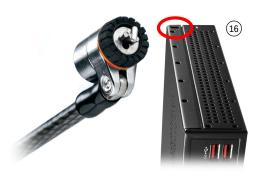
16. Hole for Kensington Lock (the lock-and-cable is not included)
