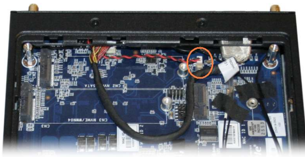
Photo: Position of the connector of the button cell battery on the mainboard with the computer housing open.
