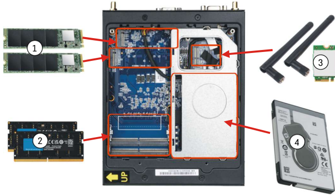
Shuttle XPC slim Barebone DS50U5 with opened chassis
