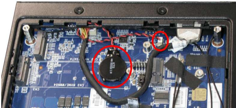
Photo: Position of the button cell battery and the connector on the mainboard with the computer housing open.
