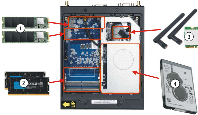
Shuttle XPC slim Barebone DS50U with opened chassis
