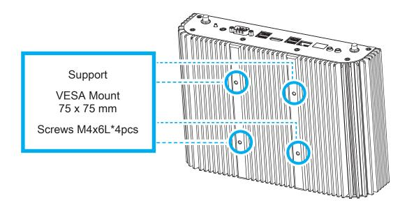
NOTE: The Box-PC can be wall-mounted using a VESA compatible 75 mm x 75 mm wall/arm bracket. The maximum load capacity is 10 kg and mounting suitable in heights of ≤ 2 m only. The metal thickness of the VESA mount must be between 1.6 and 2.0 mm.
