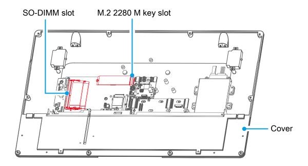
2. Install the M.2 device into the M.2 slot and secure with the screw.
