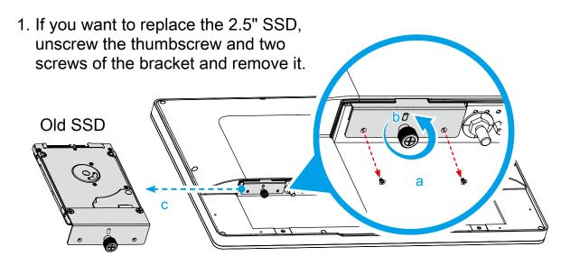
2. Unfasten the two screws (M3 x 4L) and remove old SSD.
