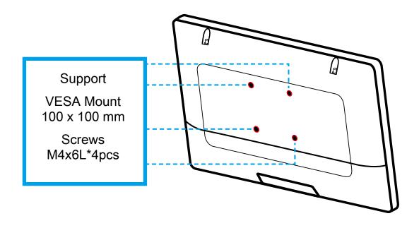
NOTE: The Panel PC can be wall-mounted using a VESA compatible 100 mm x 100 mm wall / arm bracket. The maximum load capacity is 10 kg and mounting suitable in heights of ≤ 2 m only. The metal thickness of the VESA mount must be between 1.6 and 2.0 mm.
