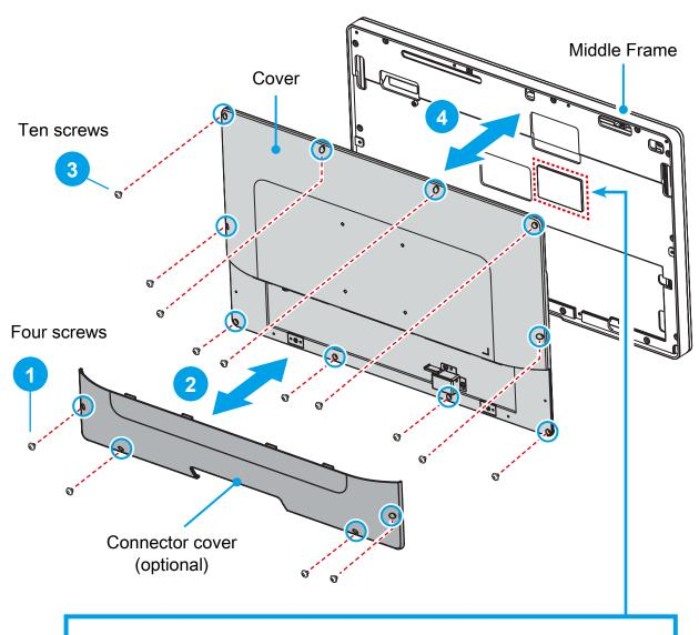
➤ If you install the M.2 SSD, please paste a thermal pad (73\*46\*5.5 mm) on the middle frame can effectively reduce its temperature.
