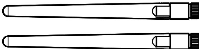
Screw the antennas on to the appropriate connectors on the back panel. Make sure the antennas are aligned vertically or horizontally to achieve the best possible signal reception.
