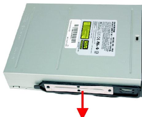
Optical drive mounting brackets
